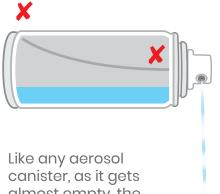
Like any aerosol canister, as it gets almost empty, the intake tube may not reach the contents if held **horizontally**.
